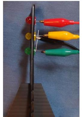
Don't clip on the battery snap connector; unlike motor outputs 1 and 2 which require the battery, the outputs A, B, C and D are powered from the computer via the micro-USB lead.
