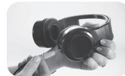
The headphone cushions can be removed and replaced with new ones. Please note that what is removed and replaced is the complete earpiece assembly including the plastic clips and the material that holds the foam on.
