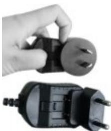
The docking station is supplied with a multi-region adaptor. The adaptor is supplied with the UK plug fitted but you can change this easily to suit any country. Press the release button and slide the UK plug out and replace it with the required plug module. Slide the plug module in until it "clicks" in place securely.
