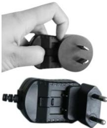
The docking station is supplied with a multi-region adaptor. The adaptor is supplied with the UK plug fitted but you can change this easily to suit any country. Press the release button and slide the UK plug out and replace it with the required plug module. Slide the plug module in until it “clicks” in place securely.
