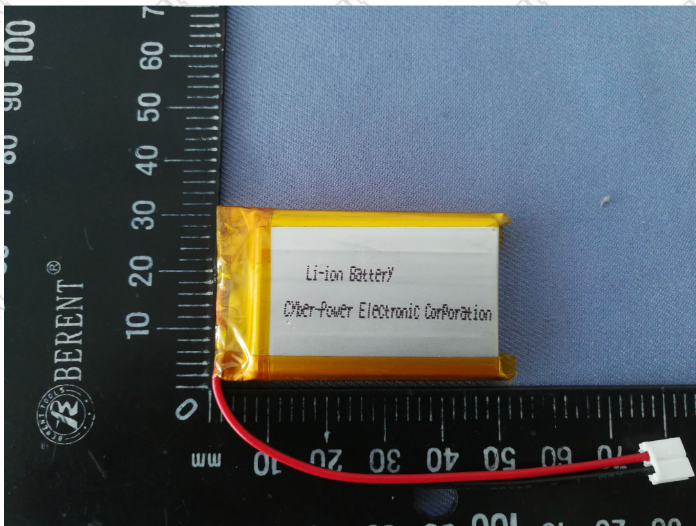
Figure 2 Overall view II of battery (电池图II)
