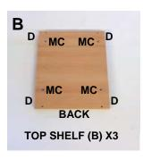
When fitting the Minifix cams (MC) please ensure the arrows on the Minifix cams (MC) are pointing to the outer edge holes.
