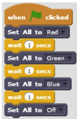
To make the Rainbow Matrix easy to use there are several blocks with predefined colours. However any one of 16 million colours can be selected using the R,G,B (Red, Green, Blue) settings. The example shown, from Key Focus 1, can be created with the 'Set All to RGB' block (left image). This can be replicated with the 'Set All to RGB' block (right image).
