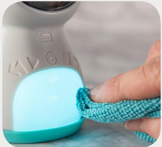
Kitt's teal cleaning cap can be hand washed and air dried if required. Please do not soak the silicone cleaning cap for extended periods or use boiling water as this can cause damage to the silicone.
