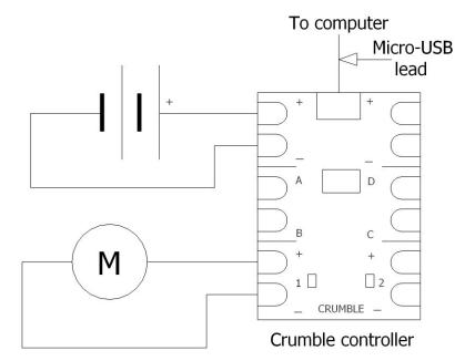
3. Add the second motor to the diagram and show how it connects to the Crumble controller. (Slide 5)
