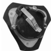
2. Insert the button cell battery into battery holder to start transmitting
